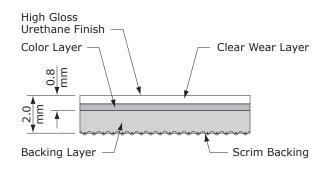
Note: M668UV differs with no clear wear layer, a thicker backing layer, and a total wear layer thickness of 0.45 mm. TEST DATA (refer to the last page for additional test information)
